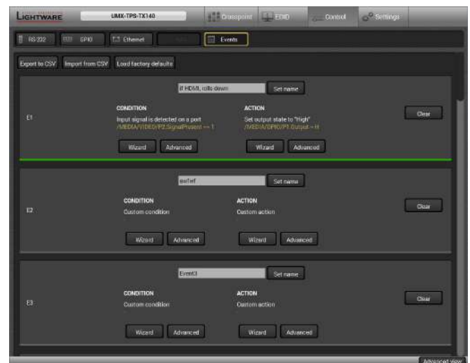
Green lines show which Event is configured and active, the rest stay grey
