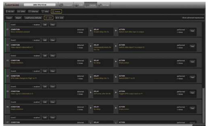
Green lines show which Event is configured and active, the rest stay grey
