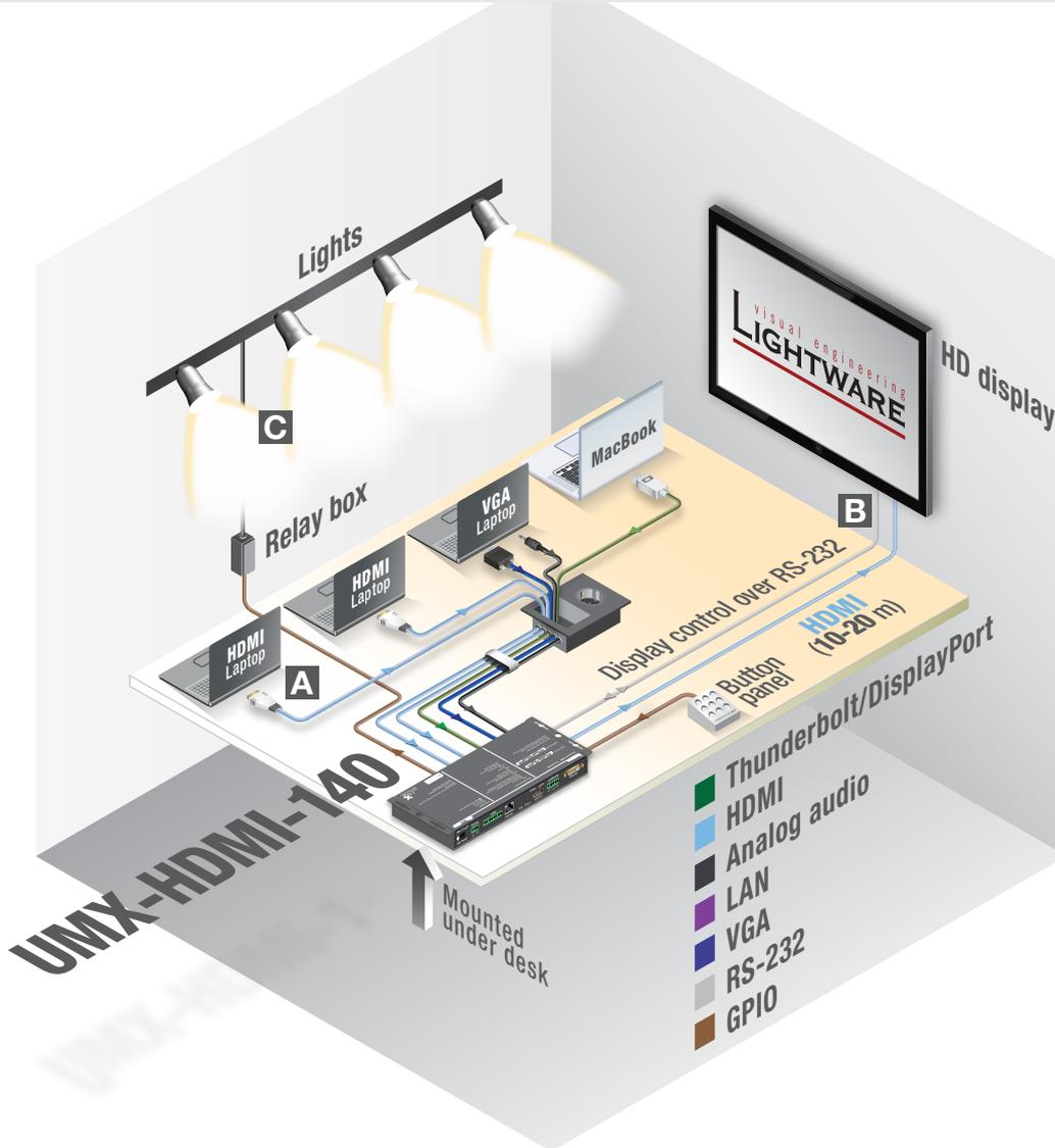
With a button panel connected through the GPIO port, the UMX-HDMI-140 can be controlled from a remote location. Input switching is available even if the transmitter is mounted under desk. In the example above there are three actions followed by a condition. When an input select button is pressed on the remote button panel, the selected input port is switched to the output, the display turns on, and the lights switch on.
