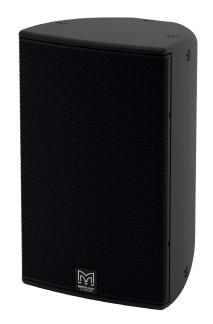
The CDD10TX is a very compact two-way passive loudspeaker system incorporating a 70V/100V transformer (with a 5-way connector) that utilises a 10" (250mm) LF/1" (25mm) exit HF Coaxial Differential Dispersion driver.
