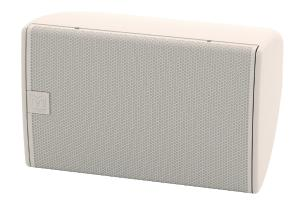
The visually-distinctive enclosure can be used in either horizontal (landscape) or vertical (portrait) orientation, with rotation of the driver easily accomplished by removing the screw-free, protective grille. The curved shape of the enclosure allows it to be surface-mounted close to a wall or ceiling by means of optional wall and ceiling brackets.
