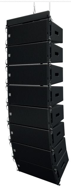
The 8" LF drivers are set back behind the walls of the HF horn, with a small volume of air in front of each driver increasing the output at the upper end of its operating range. The LF exit apertures are spaced apart horizontally to provide useful LF horizontal pattern control.
